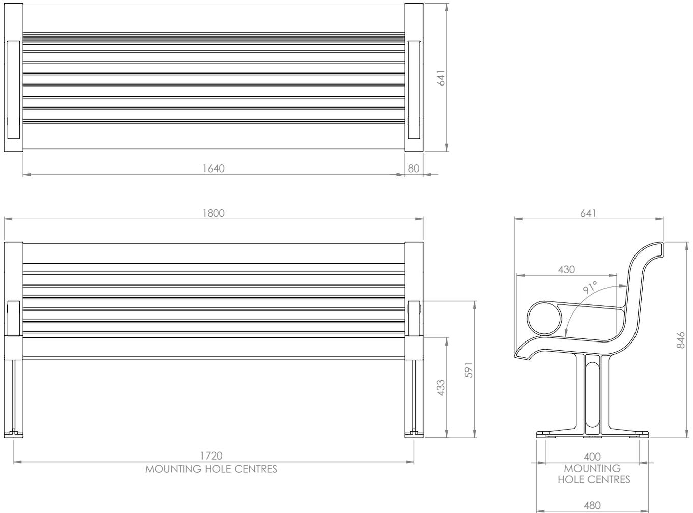
All measurements are in millimetres. Drawings are not to scale
